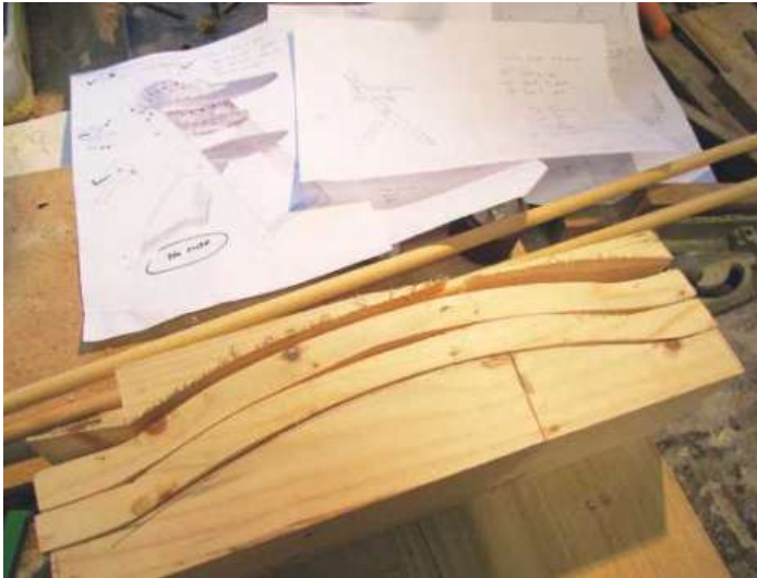
▲ Pic. 2 Bandsawing the curved seat-back was easier than steam-bending it. The better of the two pieces was ripped lengthwise to form matching top and bottom rails
